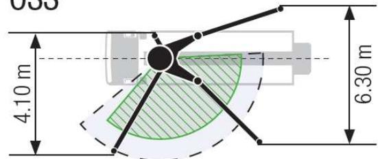
Support width based on center of support leg
