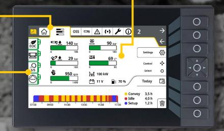
**Status indicator + color code** Each menu page offers shortcut keys for the most common functions. The shortcut keys on the EGD look the same as on the radio remote control. If the radio remote control is the selected point of operation, the shortcut keys are grayed out, but still show the current status of the function.control.
