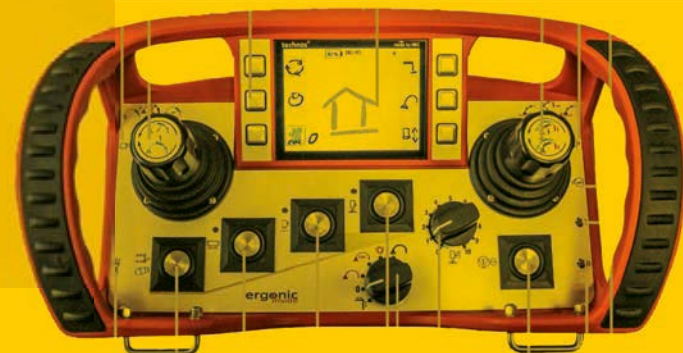
Ergonic® Inside - With the modern, ergonomic radio controls, Putzmeister machines can be operated comfortably and precisely. The graphical display shows all the important information at a glance.
