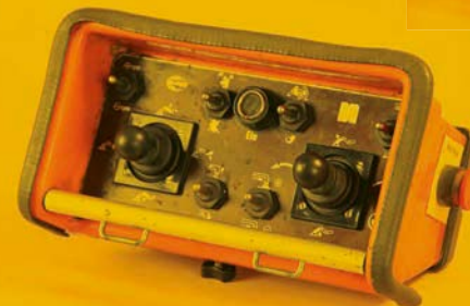
Proportional Putzmeister radio remote control from the middle of the 1980s, protected by a circulating strip, on the left for three-arm and on the right for four-arm placing booms.
