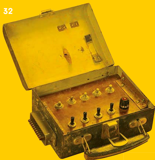
ON/OFF, BLACK/WHITE Moving placing booms evenly using black-and-white control systems required a lot of skill and experience.
