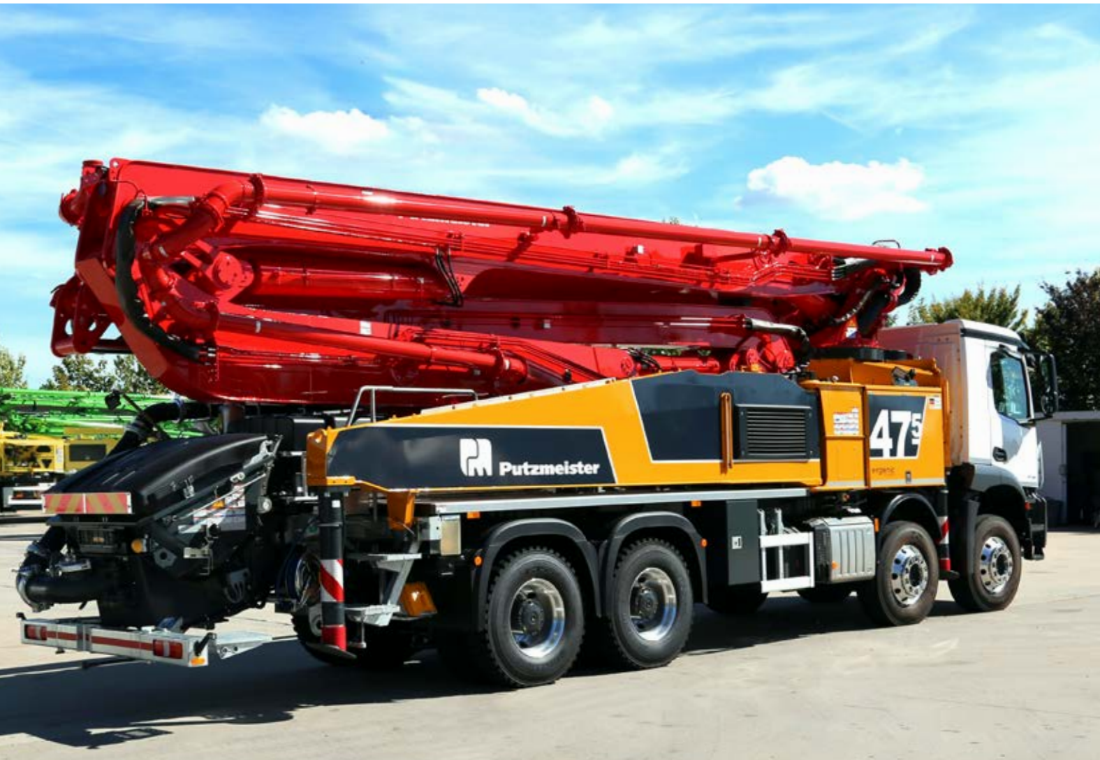
A gross weight of less than 32 t provides a high capacity for payload and functional fluids. This ensures that the machines meet country-specific licensing regulations.
