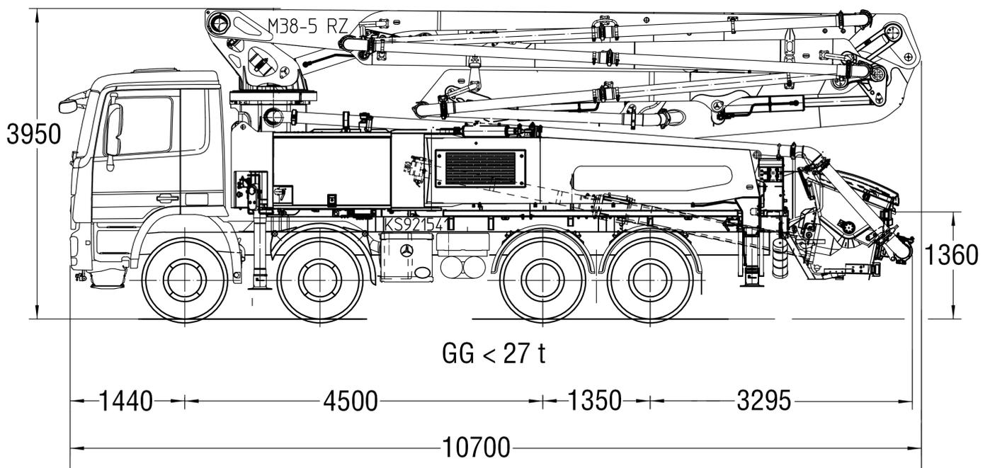
Note: Standard version. Dimensions and weights depend on truck, pump model and equipment.
