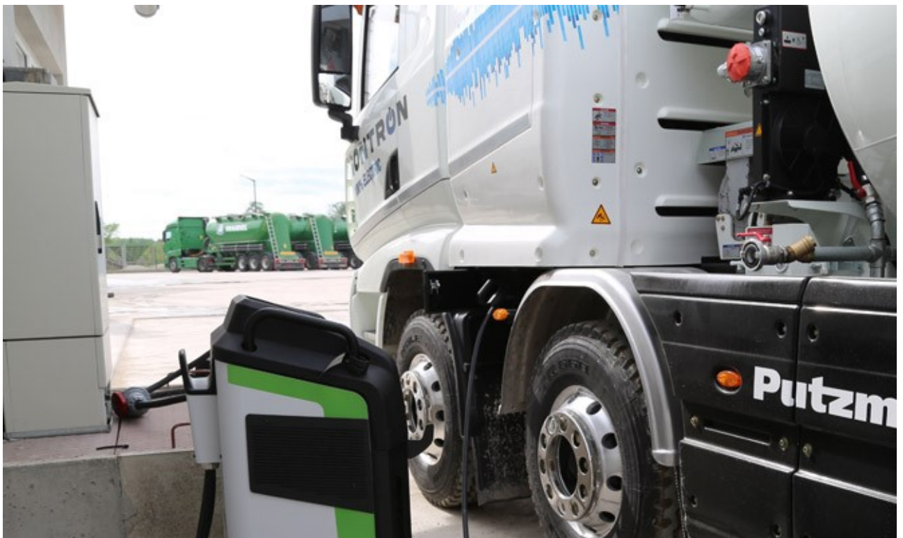
At the end of the working day, the eMixer is connected to the charging station and the battery is charged again
