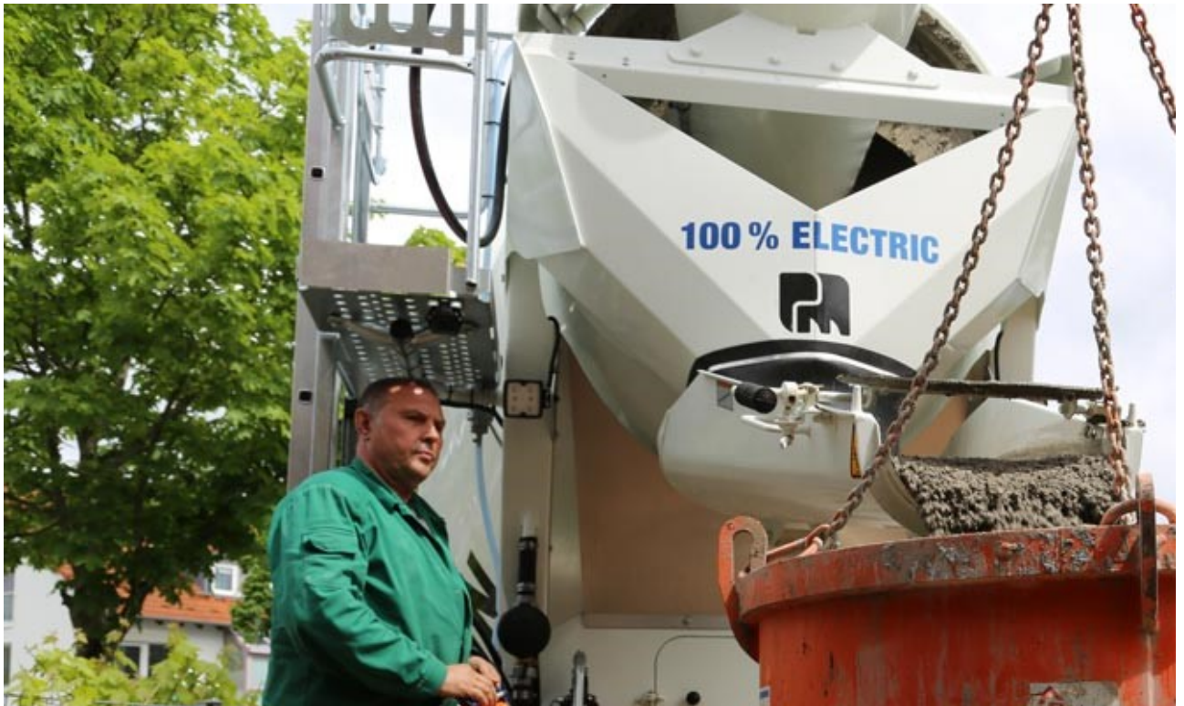
Concrete pump or concrete bucket - work is done normally with the eMixer.
