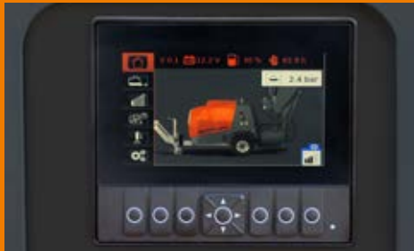
New revised operating concept: The operator can view and set all the necessary information directly from the control panel.
