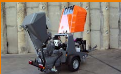
The innovative canopy concept and the removable rear section allow easy access to all important service and maintenance points
