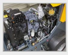
The powerful diesel engine meets all requirements of the "Stage V" emissions standard, applicable in the EU and Switzerland.
