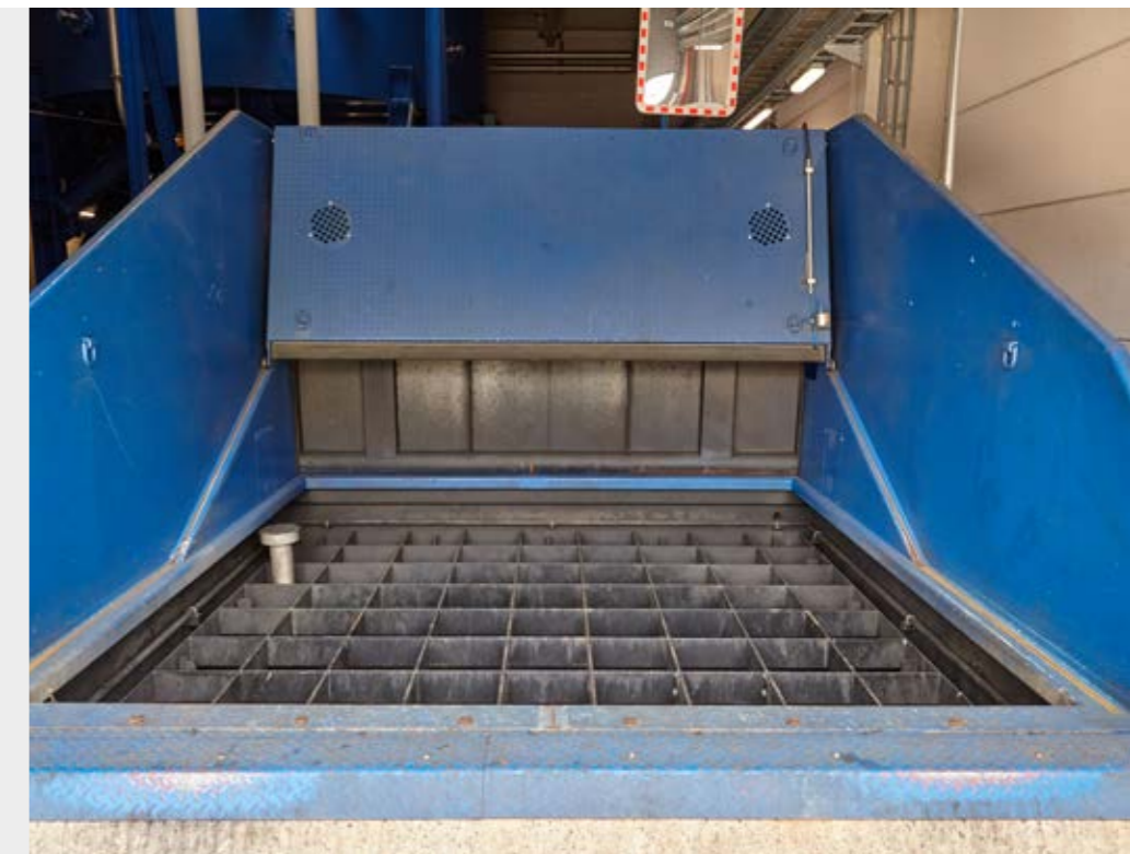
Above: Automatically controlled flaps are an important feature of receiving bunkers. Putzmeister offers a range of different variants.
