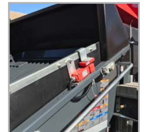
The agitator safety switch off is a worldwide standard equipment in every Putzmeister machine!
