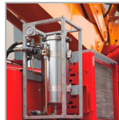
The by-flow filter is an optional fine-filter element in the oil circuit, which has a big impact on the oil quality
