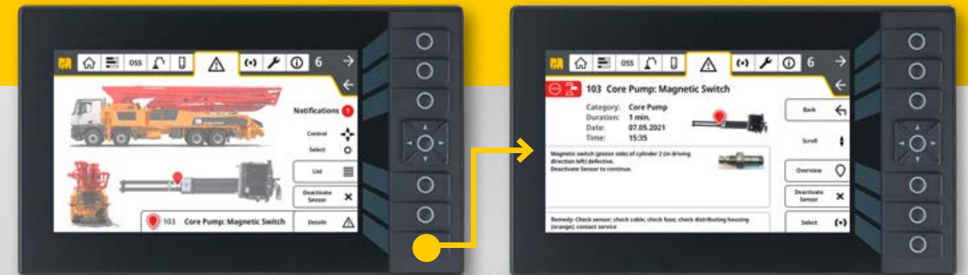
Clearly guided fault management on the radio remote control and the graphic display
