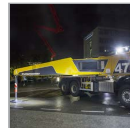
Spot lights to illuminate the four support legs make it quicker and safer to set up the machine in the dark.
