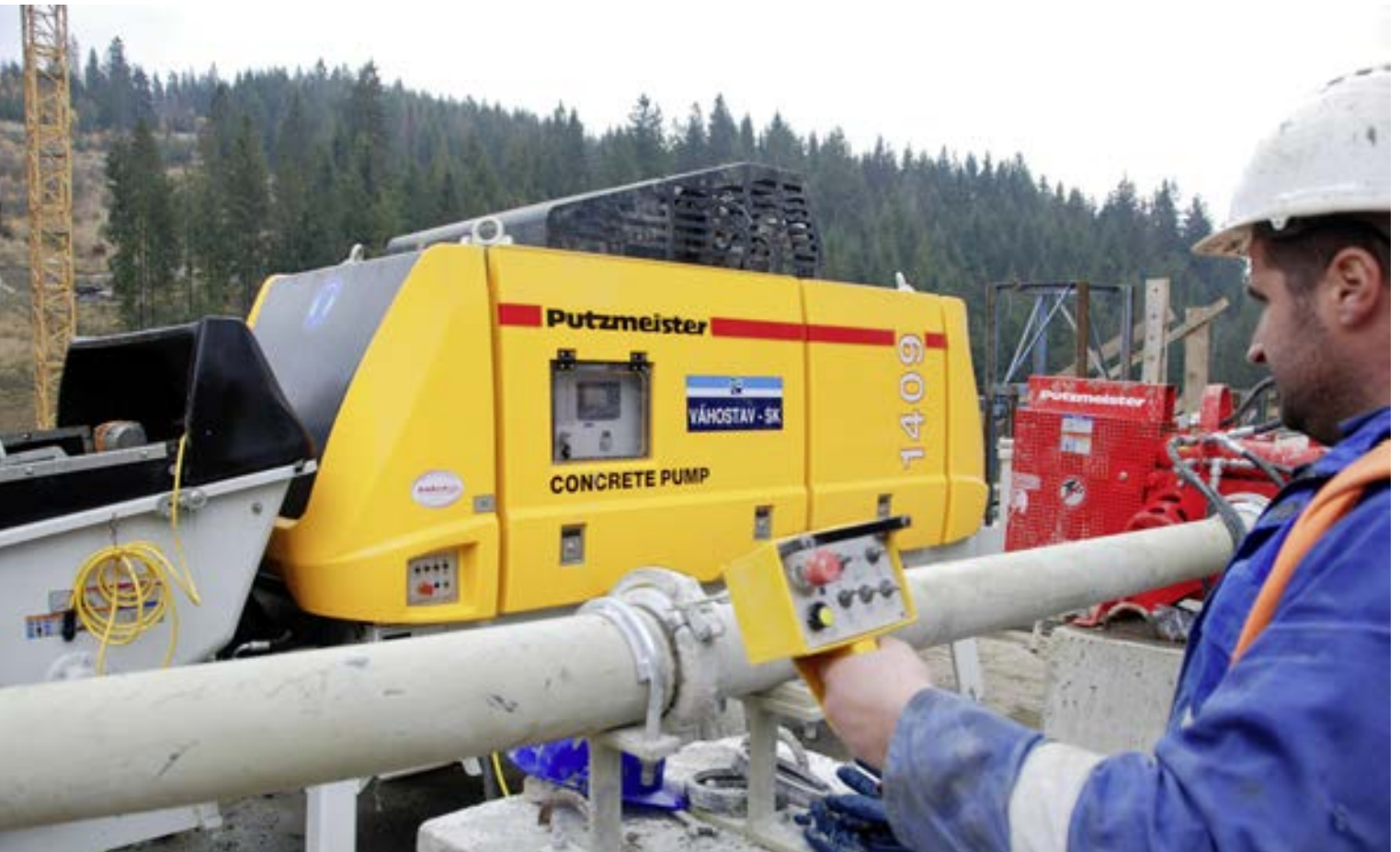
The gate valve is hydraulically driven and controlled by the stationary pump
